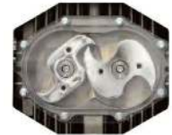
S-type pump - internal view
