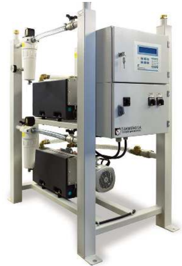
Compact Medical Vacuum Central Station according to ISO 7396-1 with: · 3 vacuum pumps 94m 3 /h · 2 filters · 1 electronic and control panel
